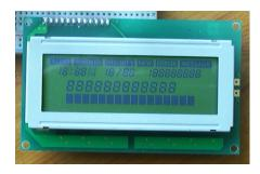
The connector (top left side) has 12 connections, numbered from the left. There are two connections at the right side marked A and K. The use is show in the table below.
