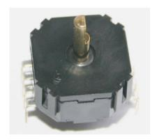
This is a small joystick switch. The pins are at a 2mm grid. If you want to use this switch in a standard 2.54 mm grid you will have to spread the pins. For use in a breadboard a I soldered the legs into the cups of a (part of) a 40-pin round-pin DIP socket.
